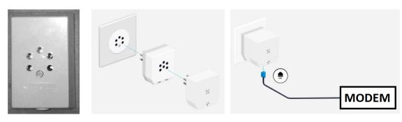
The telephony is accessible at the RJ jacks of the adapter.
