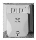
The VDSL modem shall be connected to the RJ11 jack of the pluggable splitter or of the VoIP plug with an appropriate patch cord.
